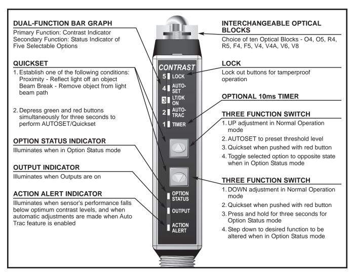
The **SMARTEYE® PRO** is not a teach mode sensor; it is an automatic sensor. It is a high performance photoelectric sensor that, after the initial setup, can be adjusted by a single push of a button. As a result, there is no guesswork on the part of the operator. Now you can throw away the screwdriver.
